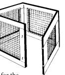
panels of wire mesh for the sides. Another design is a cube-shaped frame of two-by-fours, about 4 feet on each side, with three fixed plywood or board sides, one side a hinged door, and possibly a lid on hinges. Do not use treated or creosoted wood—it can leach toxins into your soil and compost.
