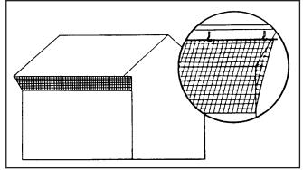
**Figure 3.** Plastic netting can be attached to a building from the outside edge of the eave and angled back to the wood siding. The insert shows one method of attachment using hooks and wooden dowels.
