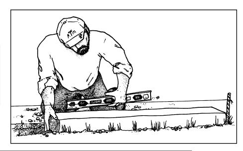
Secure the first row of timbers by driving a piece of rebar through a predrilled hole and into the ground at a 20-degree angle. Secure subsequent rows with three or four spikes or pieces of rebar per timber. Make sure spikes extend well into the timber below.
